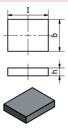
$\begin{array}{ll} b & = 6 \\ h & = 2 \\ I & = 7.5 \\ \text{Nominal adhesive forces} = 8 \\ \text{Weight in g} & = 1 \end{array}$
